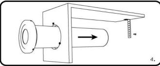
4. Push the cup dispenser to the counter hole. Useend screw to hold the tube.
