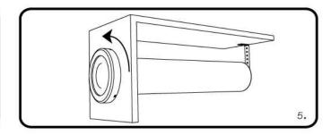
5. Aim the key hole of front plate to the tapping screw head. Rotate cup dispenser counter clockwise to lock.
